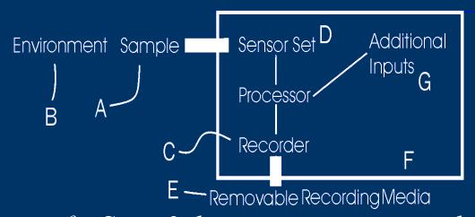
The purpose of a Signa2 device is to acquire and record a sample (A) of the environment (B) in such a manner that the stored recording (E) is verifiable as an authentic representation of the sample (A) and has not been altered from point of acquisition in the environment (B). Authentication information generation capability must be indigenous (F) to, and inseparable from, the device.
